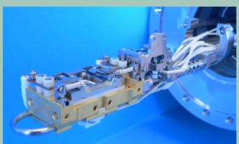
Power feedthrough contacts and temperature readouts
